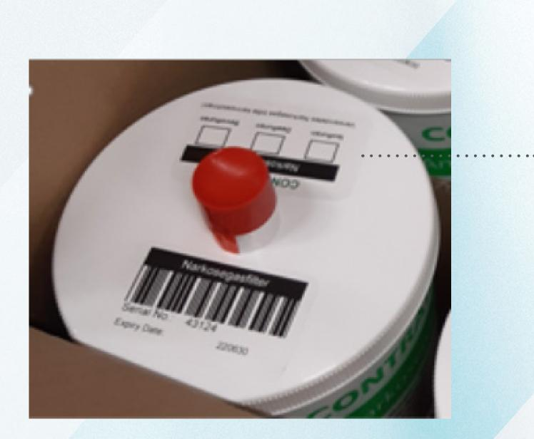
To help optimise the gas recycling process, the correct box(es) should be ticked on the sticker on top of each canister, indicating which gas (or gases) are contained within.<sup>1</sup>
